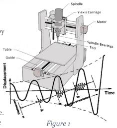
Chatter results from the momentary separation of the tool and workpiece and the immediate banging back into contact. It is a danger signal of impending possible chipping or fracture.
