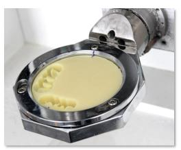
*Example of vibration enducing fixturing: fixture held on only one end.*
