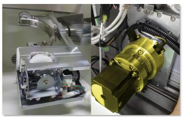
*Figure 2 Comparison of rotary reduction drives between two different dental machining centers.*
