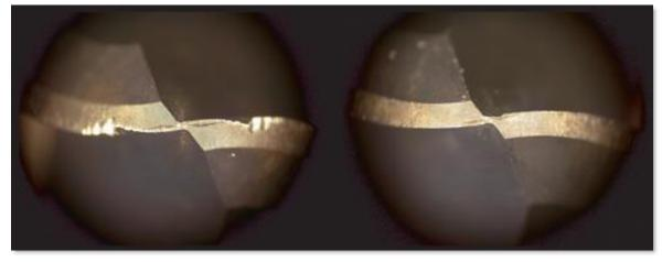
Compare image of worn tool on the left with a new, unused tool on the right.
