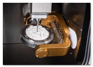
*Example of proper fixturing: workpiec & fixture held securely on both ends.*
