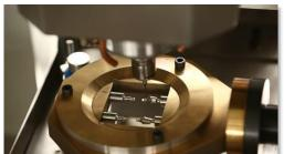
Example of vibration enducing workholding : workpiece & fixture held on only one end.
